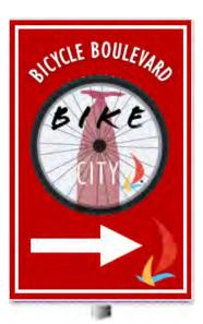
Indicates where a bikeway turns from one street onto another street. Can be used with pavement markings
