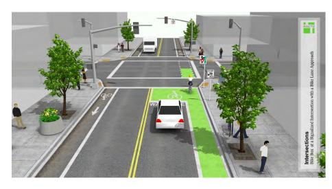
Green-painted rectangles (with a white outline) at intersections that provide a safe refuge for bicyclists to either cue ahead of cars or to make a two-stage turn. Bike boxes help increase safety for bicyclists by reducing right-hand hooks by cars and by helping bicyclists navigate tricky intersections, such as where there are streetcar tracks.
