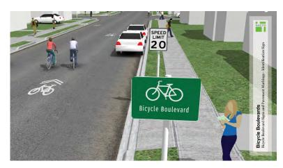
Bicycle boulevards are streets with low motorized traffic volumes and speeds, designated and designed to give bicycle travel priority. Bicycle Boulevards use signs, pavement markings, and speed and volume management measures to discourage through trips by motor vehicles and create safe, convenient bicycle crossings of busy arterial streets.
